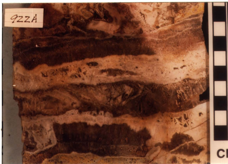
Figure 39. Hand sample 922 collected in the west pit, Hill 1 (Plt. 5). Note rhythmic manganiferous calcite-dominant versus chalcedonic quartz-"snowflake" calcite dominant banding. Note Stage IV breccia fragments near the wall rock edge (a) that shows Stage V quartz cementing. Scale in cm.
