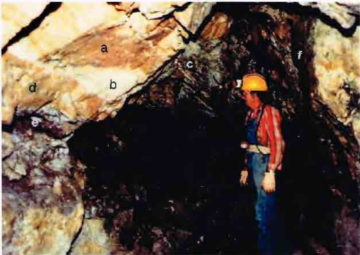
Figure 16. Underground view looking south-southwest along the main drift on the 3300-foot level of Shaft No. 2 (Hill No. 2) of the Telegraph Mine. The west dipping attitude of the main breccia-vein is evident and all stages of mineralization are exposed. Light tan Stage IV breccia (a) hosting white Stage V veins (b) occupy the zone’s central exposure, with greenish-grey Stage III breccia developed along the footwall and hanging wall (c). Note large Stage III clasts included within Stage IV breccia (d). Manganese-oxide-rich Stage VI fissure veins occupy both re-opened shallow structures within the main zone (e) and high-angle structures in the hanging wall (f). (photo from Lange, 1988, Figure 28.)
